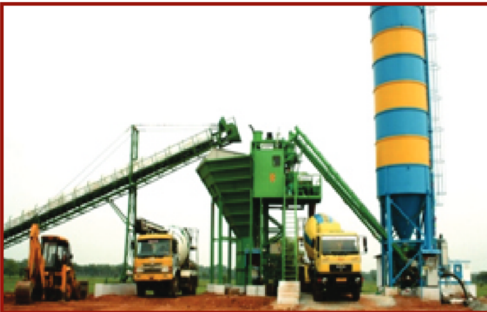
RMC PLANT TWIN SHAFT & PAIN MIXER
